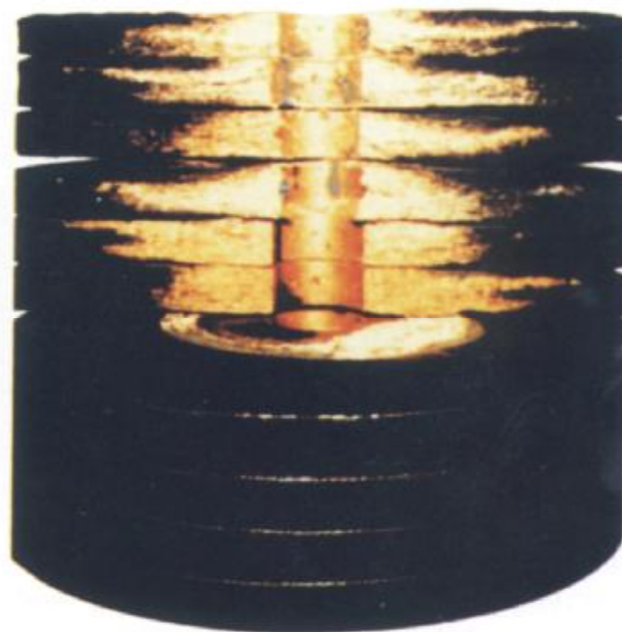
Cut-down in used CJC Filter insert - Type HDU 27/27
